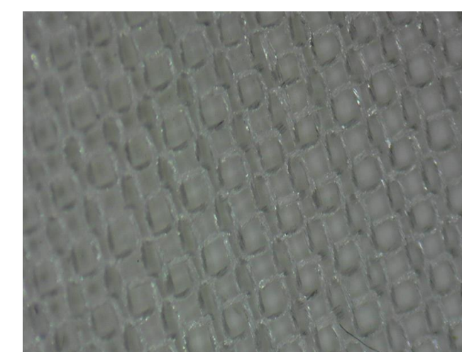
Fig 7. single layer of silk before “welding” with density of 0.1131 g/cm 3
