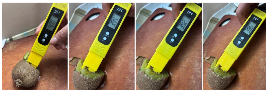
Figure 2 Process of Detecting Fruit pH Value with a Commercially Available Household pH Pen
